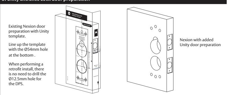
• Use the Unity Entrance lock installation template to prepare the door as shown above, which includes 2 by Ø54mm holes and 4 by Ø10mm holes.
